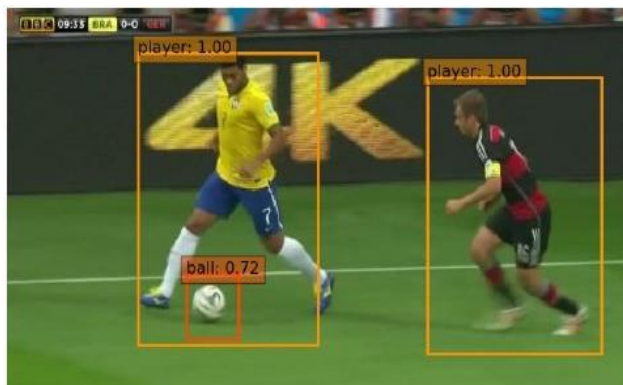
Fig.5 Detection of object by SSD with confidence score
