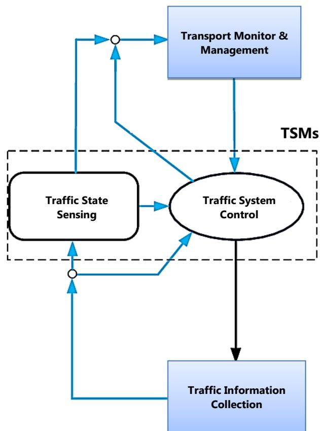
**Figure 1.** The architecture of an Intelligent Transportation System
