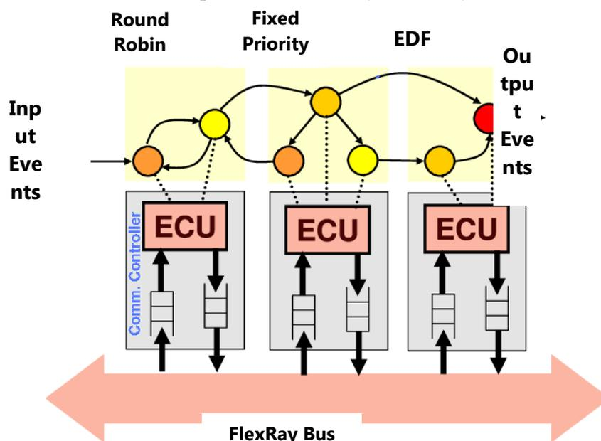
**Figure 4.** Network Configurations of ECUs
