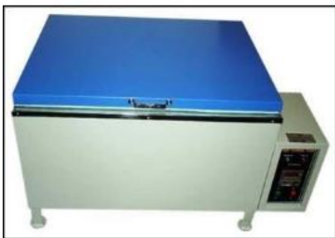
Fig.2. Accelerated curing tank used in laboratory for concrete testing
