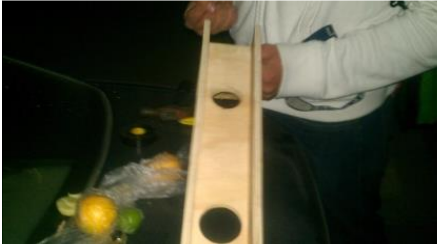
Figure 4. Manufacturing process of the three holes for detecting the dimensions of the oranges
