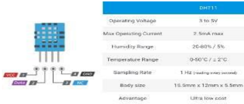
Figure 8. DHT11 Technical Specifications
