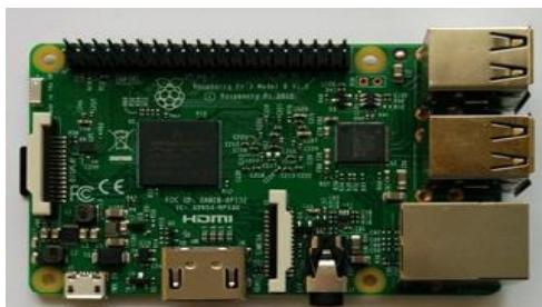
Fig.2. Raspberry pi 3 model
