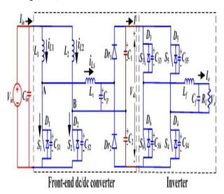
A zero-voltage switching (ZVS) and ZCS operated current-fed CL-resonant dc/dc converter. A current-fed bidirectional full-bridge converter based inverter. The proposed converter achieves ZCS of the primary switches and ZVS of the secondary devices with natural device voltage clamping.
