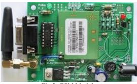
Fig.2. GSM Module
