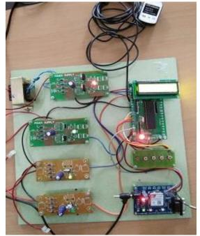
Fig.3. Underground cable fault distance locator
