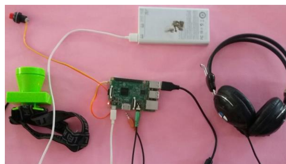
Fig.4. Snapshot demo system including three functional components for camera, raspberry pi and headphone
