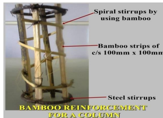
Fig.5. Bamboo reinforced column
