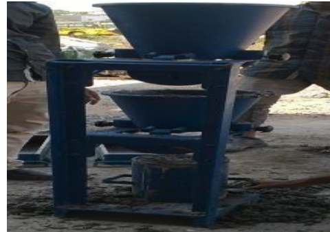
Fig.3. Compaction Factor Test
