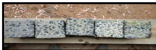
Fig.7. Cubes after exposure to H 2 SO 4
