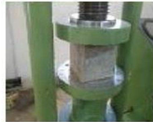
Fig.2. Test of cubes for compressive strength
