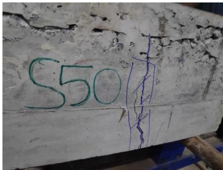
Fig.6. Failure Mode of S1 (50mm)
