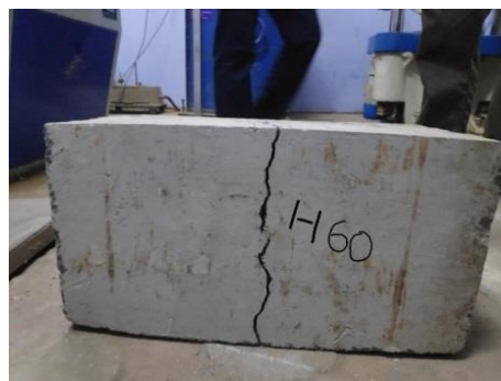
Fig.8. Failure modes of H2 (60mm)
