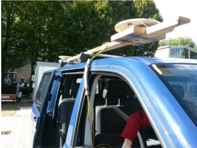
Fig.3. The GPS-PPP equipment mounted on the vehicle
