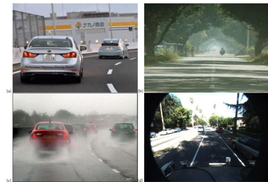
Fig.6. Various challenges in lane detection. [a] A vehicle occluding nearby lane [b] Presence of shadow [c] Rainy road [d] Extreme illumination on left side of image
