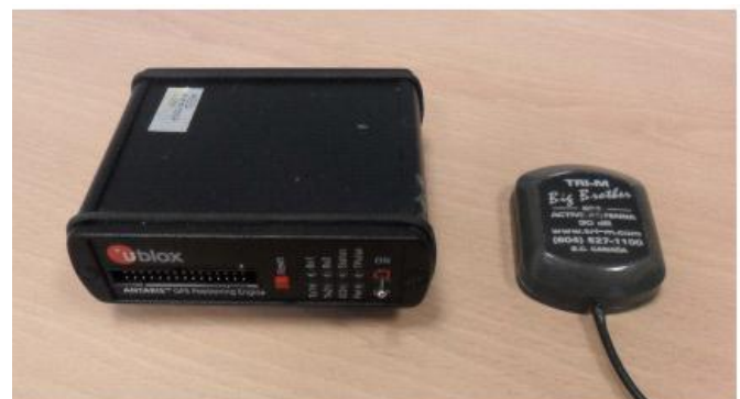
Fig.2. The u-blox TIM Lp single frequency receiver evaluation kit (left) and Tri-Big Brother patch antenna
