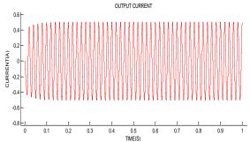
This is the output current waveform of single stage boosting inverter with trap CL filter. Pure sinusoidal waveform is produced in the output waveform. X-axis is represented as time in seconds and Y-axis is represented as current in amperes.
