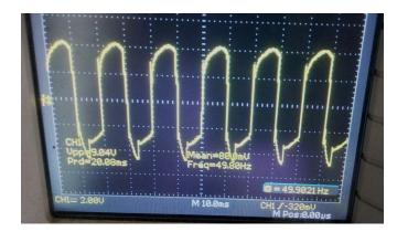
This is the output voltage of single stage boosting inverter with trap CL filter for photovoltaic application. Output voltage is greater than the input voltage due to boost converter. Efficiency is improved by trap CL filter.
