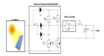
MOSFET switch is a three terminal fully controlled switch. It has gate, drain and source. It is used to improve the switching speed and dynamic response under less power. MOSFET switch S1 and S4 turns ON then switch S2 and switch S3 is turns off. Then switch S1 and switch S4 turns OFF and so switch S2 and switch S3 turns ON.
