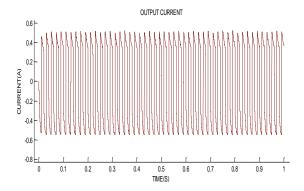
This is the output current waveform of single stage boosting inverter. Approximately 0.3A is produced in single stage boosting inverter. Current value is depend upon the load variation.
