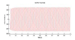
This is the output waveform of single stage boosting inverter with trap CL filter. The output voltage is 230V. It is high compared to the without trap CL filter. Pure sinusoidal waveform is attained in the output waveform. X-axis is represented as time in seconds and Y-axis is represented as voltage in volts. Voltage is varied with respect to the time.
