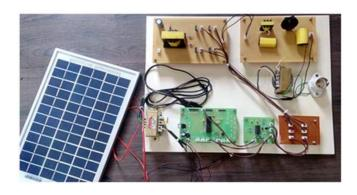
Coupled inductor is used to reduce stress across diode and reduce the conduction losses. MOSFET switch is used in the boosting inverter. Ferrite core is used in the coupled inductor and it is operate in high frequency and low losses. Capacitor and diode is used for boosting inverter operation.
