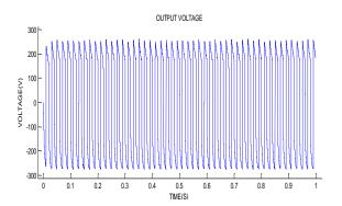
This is output voltage of high gain single stage boosting inverter. Harmonics is involved in the single stage boosting inverter so pure sinusoidal waveform is not produced. Approximately 170V is produced in the boosting inverter. Efficiency drop is occurred due to some stress and harmonics.
