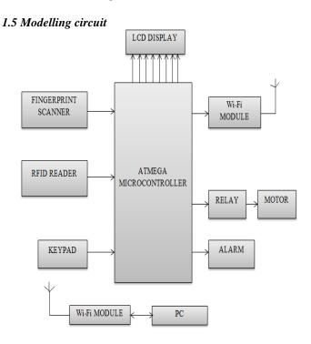
Fingerprint scanner is an electronic device used to capture a digital image of the fingerprint pattern. The captured image is called a live scan. This live scan is digitally processed to create a biometric template which is stored and used for matching. Many technologies have been used including optical. Capacitive, RF, thermal, piezo-resistive, ultrasonic, piezoelectric, MEMS.
