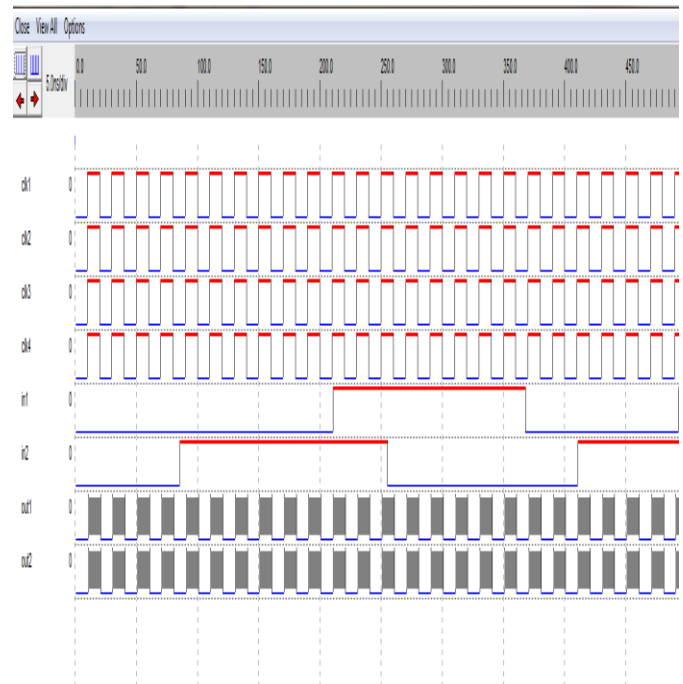
Fig.5. Simulation Output of 3- Bit Comparator
