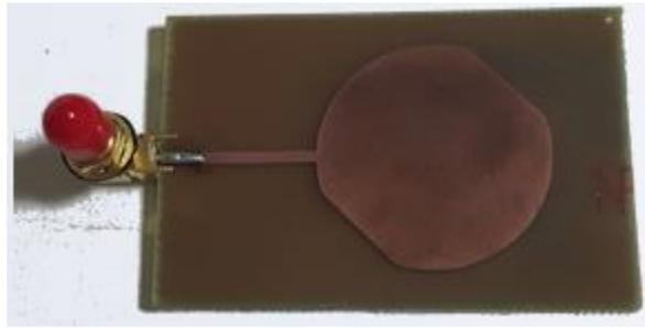
**Fig.1** Sample model of Circular Dipole Antenna
