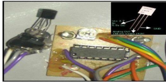
Fig.2 Body Temperature Sensor & Its Circuit
