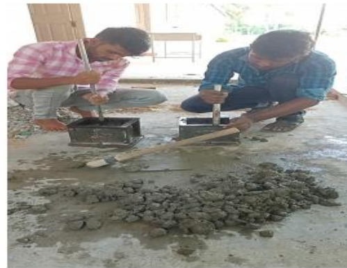
Fig.3. Compaction of concrete by tamping rod
