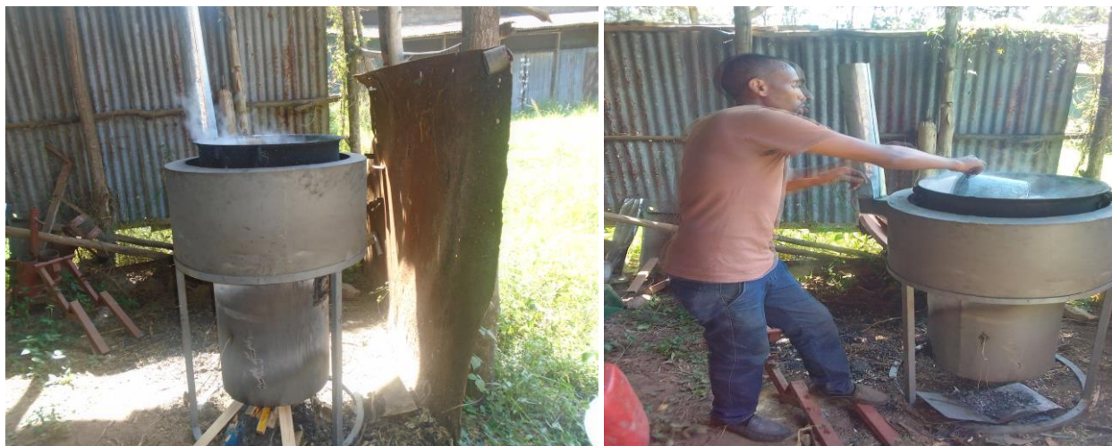
Figure 2.3: WBT of Institutional Bio-char Rocket Stove
