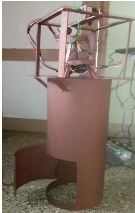
Figure Mechanical Setup of Bore well with 2 DC motors
