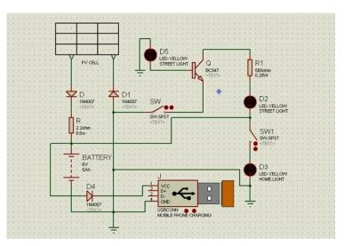
Generally in photovoltaic (P.V) system in between solar p.v module & battery there is a C.C.U (Charge controller unit) [8]. In that case we used 2 pieces of diode for controlling the circuit. But if it has to be worked above 10w.p. and 12 volt photovoltaic system then the charge controller is needed to be replaced for controlling the circuit.
