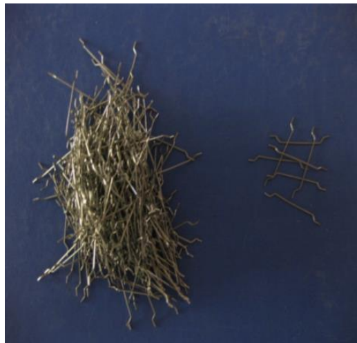
Fig: Hooked end fibers
