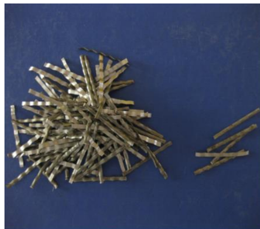
Fig : Crimped fiber
