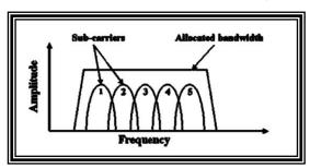
An OFDM transmitter accepts data from an IP network, converted and encoded the data prior to modulation. The inverse fast fourier transform (IFFT) transform the OFDM signal into an IF analog signal, which is sent to the RF transceiver. The receiver circuit reconcept the data by reversing this process OFDM actually provide better link and communication quality.
